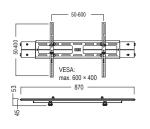
Monitor can be mounted straight or at an angle of 10° max.
